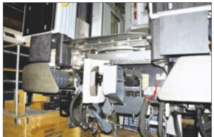
The outer ends of the carriages at each end of each rake are to be fitted with combined Type SA3 automatic and UIC screw couplings. This couplings, necessary for use on the 1,520 mm gauge network, are produced by Voith (see R 4/14, p. 52). Voith also produced the high impact absorption buffers fitted to this batch of carriages. The inter-car couplings are only of the UIC screw type.
