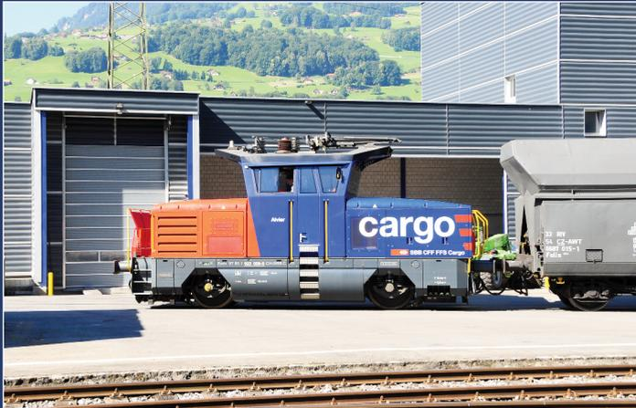
**Team Centres are responsible for collecting and delivering wagons to clients, and at these centres Class Eem 923 hybrid shunters and Class Am 843 diesel shunters are used. This photo shows Eem 923 009 shunting at Flums on 16 August 2013.**
