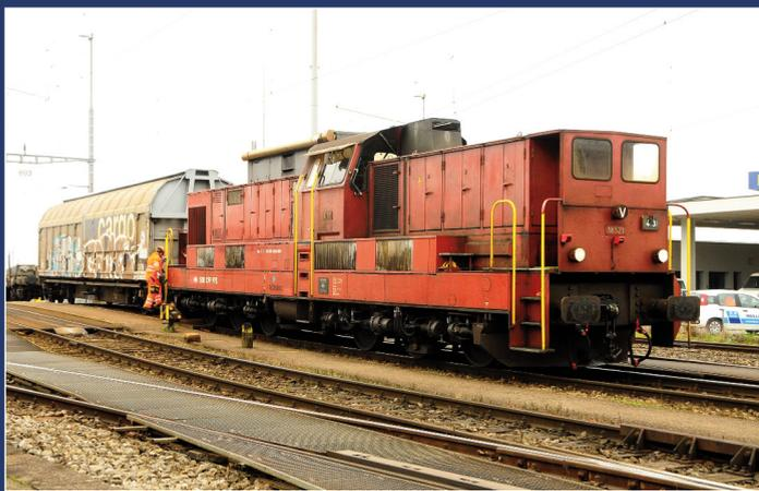
Two Class Am 6/6 heavy duty diesel shunter, remote-controlled from a control centre, are used on shunting humps at Zürich-Limmattal marshalling yard. This is Am 6/6 18521 on 28 October 2016. The Class Am 6/6s are Co'Co' locomotives built in 1976 by Thyssen Henschel and BBC, and in 2018 will be replaced by new Prima H4 electro-diesel shunters.
