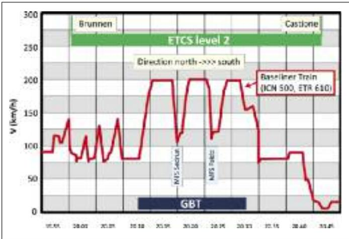
**A graph showing the progress of IC services (red line) through the 57 km Gotthard Base Tunnel. On 4 November 2016 over the high speed pointwork at the crossovers at Sedrun and at Faido (15 km from the southern portal) it was necessary to reduce speed to 120 km/h while authorisation of the pointwork at these locations was in progress. By mid-November the limit was raised to 160 km/h, and immediately before authorisation on 5 December 2016 it was lifted to the line speed of 200 km/h.**
