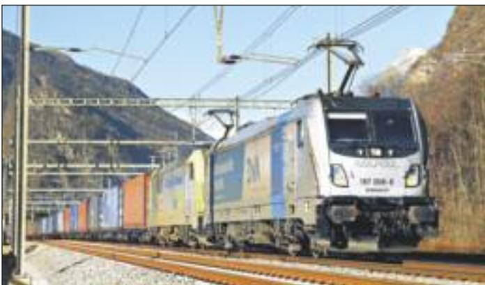
**On 1 December 2016 BLS's TRAXX 187 008, on hire from Railpool, leaves the southern portal of the GBT.** This class received a new operating permit from BAV for the GBT line on 28 November 2016, following the upgrading of their on-board EBI Cab 2000 ETCS. Those 187s which have not yet been subjected to the upgrade can still use the tunnel, but not in the position of leading locomotives.
