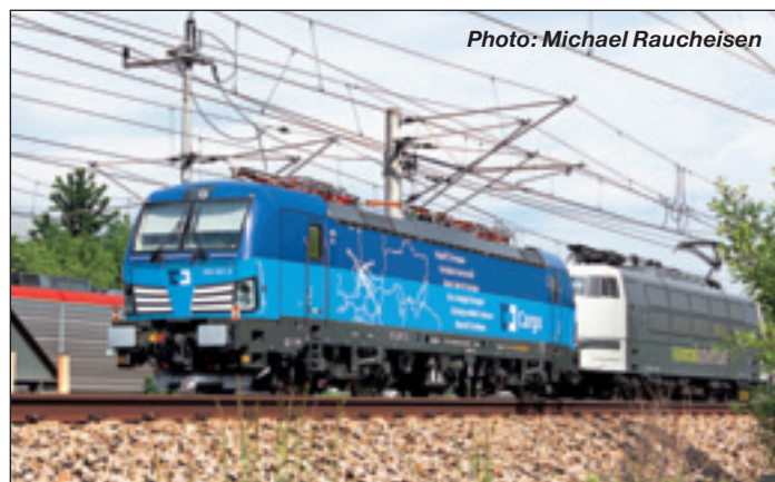
This is PKP Cargo's EU46-512 undergoing its first electrical test, with power on to activate all on-board systems, as part of commissioning, which requires that all the systems have to be approved.
