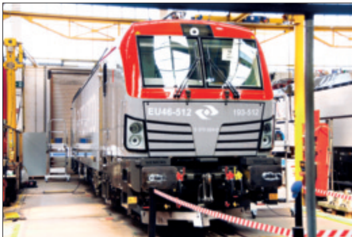
This is PKP Cargo's EU46-512 undergoing its first electrical test, with power on to activate all on-board systems, as part of commissioning, which requires that all the systems have to be approved.
