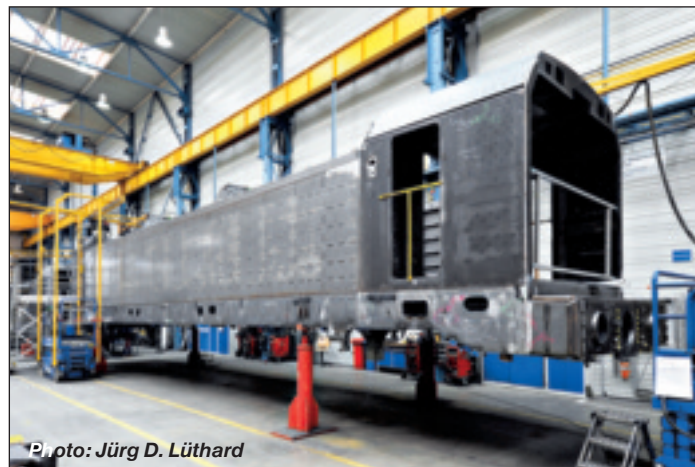
Here the bodysheaths are being welded in a different work station, before being moved to the bodysheath stockpile.
