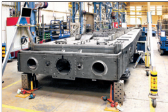
The main frame of another Vectron is born. This is the steel workshop, where welding and assembly of main frames take place.
